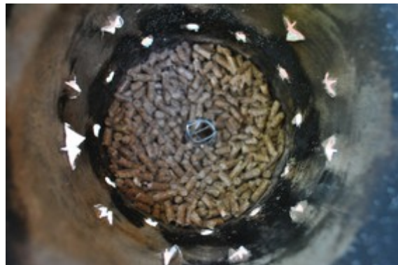
Figure 5. The cone-like shape can be seen in its position in the bottom center of the fuel column.
