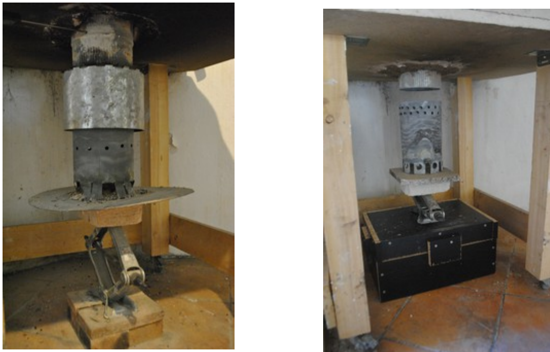
Figure 7. Holding the stove with the jack. Objects below the jack (like the black box) can be added depending on the total height of the stove
