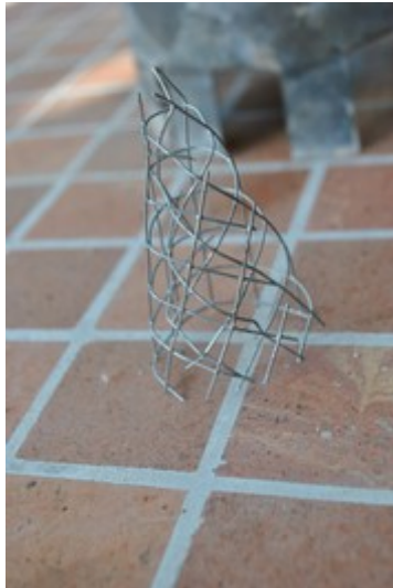
Figure 4. Cone-like shape to improve air flow during the char burning phase
