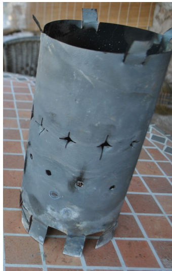
Figure 2. TLUD Reactor. Diameter: 15cm. Total length: 29cm. Fuel Height: 18cm. Primary air entrance is at the bottom. Secondary air entrance are 8mm holes rings, one at 9cm from the bottom of the fuel, the other at 14cm.
