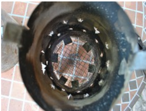
Figure 5. The cone-like shape can be seen in its position in the bottom center of the fuel column.
