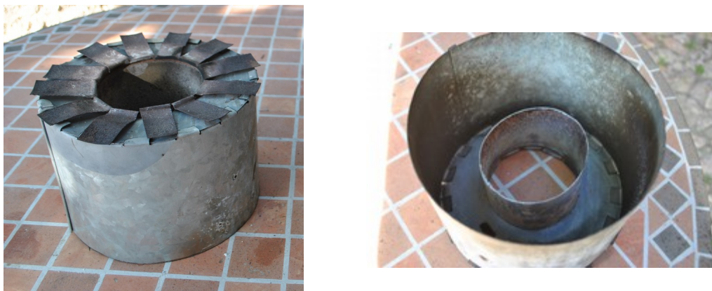
Figure 3. TLUD Combustor. Exterior diameter: 20cm. Interior diameter: 10 cm. Total length: 14 cm. Total length internal chimney: 8cm. The interior chimney
